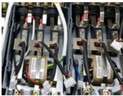
On line soft starter which working no need by pass contactor
